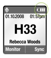
If the charging unit is removed from the inspiro, the segments in the battery symbol show the actual capacity.
