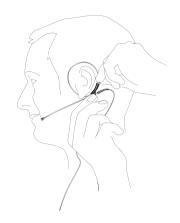
c) Hold the iBoom with one hand and slightly pull the black lever with the other hand to reduce the diameter of the ear loop until the iBoom holds securely.
