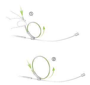
Open the loop carefully and attach the iBoom to the left or right ear.
